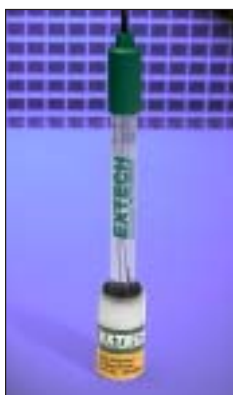
pH electrodes (except model 60120B) come with storage bottle with solution to prolong electrode life.
